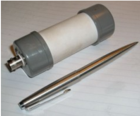
Fig. 5 De mini-whip in (witte) PVC-pijp
